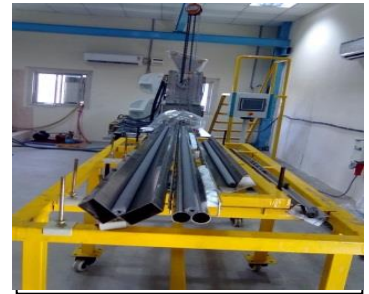
Extrusion of SiC tubes
