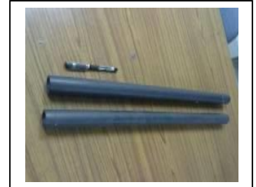
700 mm long sintered SiC tubes
